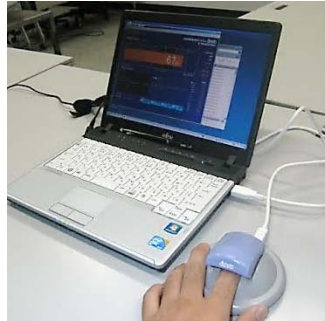
Figure 3. Portable blood vessel age measuring system (U-medica Artett2 PDU-M200)
